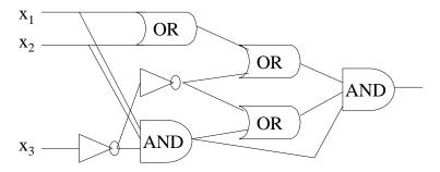
In the above circuit, can you find values for X1, X2, and X3 that makes the output 1? Apparently we may need to simply try all the (exponential) possibilities until we find a satisfying assignment. In this case the assignment 1,1,0 makes the output 1.
