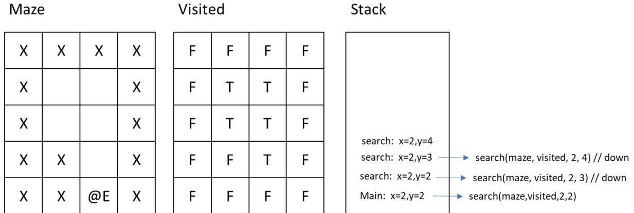
The (x,y) coordinates stored on the call stack contain the locations we need to move to in order to reach the goal. If we simply output these coordinates (or the board with the @ at these coordinates) as the recursive search function exits a found exit, then it will output the sequence of mazes to reach the exit.
