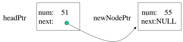
We just built a linked list consisting of two elements! The end of the list is signified by the *next* field holding NULL.
