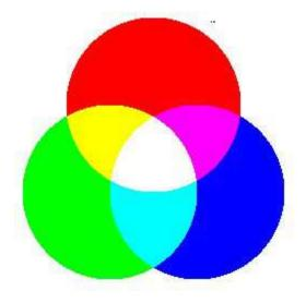
The color wheel below shows more ranges of color for different RGB values. Once again, for our case, the values range from 0-1 instead of 0-255 so substitute 1 for 255, and 0.5 for 127, etc.
