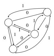
We can make the transformation in polynomial time. If we run TSP on this problem, then if there is a Hamilton cycle in the original graph G, the TSP must return a path of total cost 0 (not using any other links we added and we formed a cycle) on graph G'.
