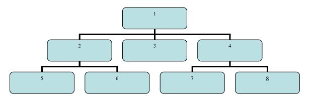
Sometimes we can stop the algorithm if we are looking for a particular element, but the general BFS algorithm runs through every node.
