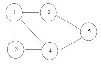
The **degree** of a vertex in an undirected graph is the number of edges that leave/enter the vertex. The degree of a vertex in a directed graph is the same,but we distinguish between in-degree and out-degree. Degree = in-degree + out-degree.
