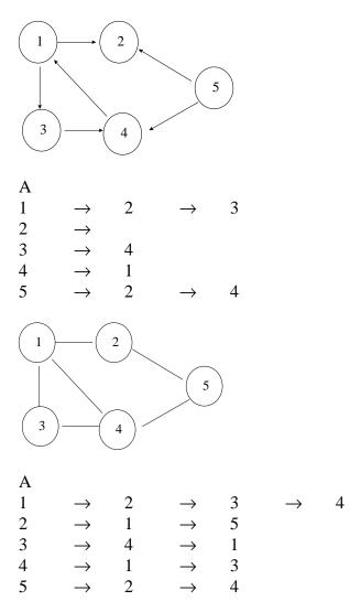
The sum of the lengths of the adjacency lists is 2|E| in an undirected graph, and |E| in a directed graph.
