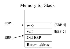
We can now refer to the local variables via [EBP-2], [EBP-4], or even via absolute address if we wish. When the procedure exits, the first thing we do is move EBP to ESP, which has the effect of popping off all the local variables we allocated:
