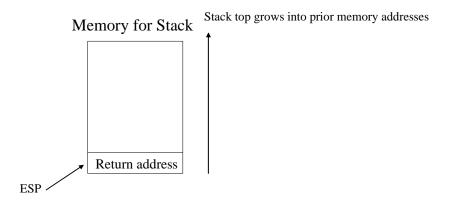
The first thing we do is push the existing EBP value on the stack, which decrements the ESP by the size of the EBP register:
