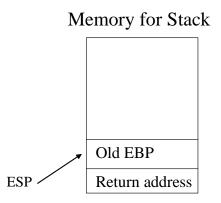
Next we copy the value of ESP into EBP, which makes EBP point to the same thing as ESP:
