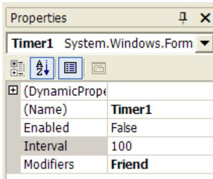
The timer is inactive if Enabled is set to False. Once Enabled is set to true, the timer behaves like an alarm clock. It starts counting down, using the value in the Interval property, until it reaches zero. The value stored in the Interval property is in **milliseconds**, not seconds, so if you wanted a countdown of 5 seconds then you would store a value of 5000 in the Interval property.
