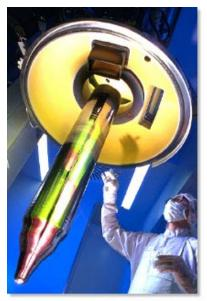
This ingot is sliced with a diamond saw into thin wafers. The transistors are then "etched" into the wafer using a lithography process similar to photography. Masks are laid over the wafers, ultraviolet light is shone through the mask, and the chip is built up in layers on the silicon wafer. The entire process takes about three months and the end result is multiple chips etched onto a single wafer. Here is a cross-section of a sample wafer:
