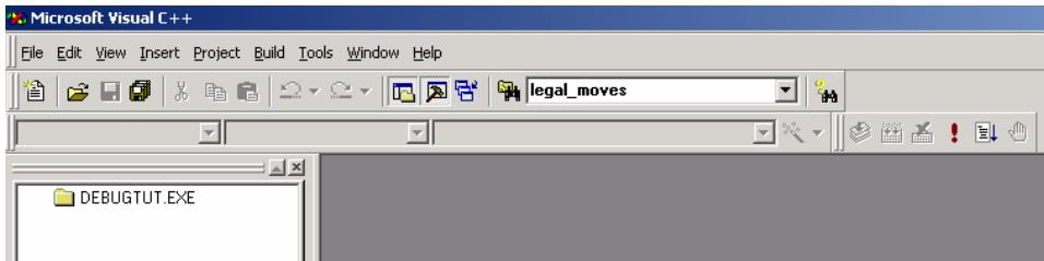
Not a very helpful screen. But if you press F11, or select B)uild, Start D)ebug, S)tep Into, then this will start the debugger and allow you to step through the program:
